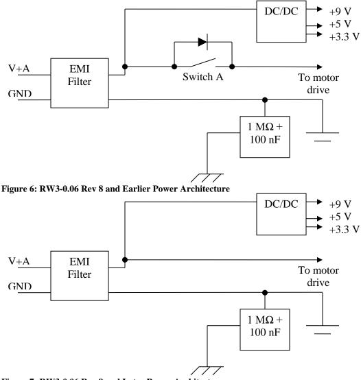
Figure 7: RW3-0.06 Rev 9 and Later Power Architecture
