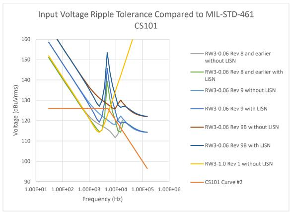
Figure 8: Allowed Bus Voltage Ripple, Sustained
